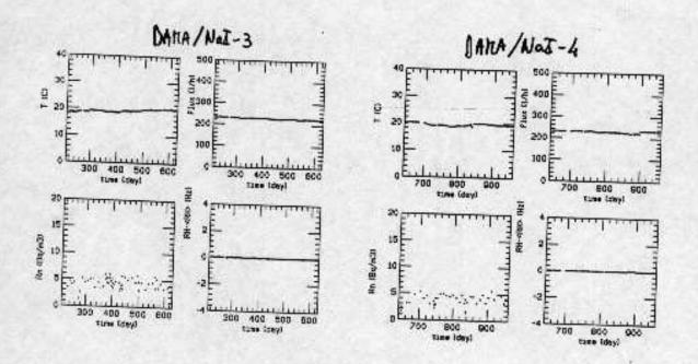
Sizeable temperature variations could cause (PSA not used!) only small light response variation: average slope of the light output ≈ -0.2%/oC in our operating temperature range.
